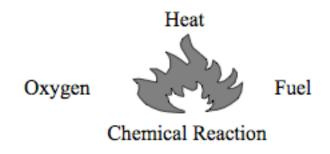
The first component of the tetrahedron is fuel. Fuel can be any combustible material such as: solid (such as wood, paper, or cloth), liquid (such as gasoline) or gas (such as acetylene or propane). Solids and liquids generally convert to gases or vapors before they will burn. Another component of the tetrahedron is oxygen. Fire only needs an atmosphere with at least 16% oxygen.
